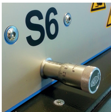
The classic micrometer allows you to easily set the crimping diameter.
