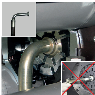
The S6 series allows to crimp short 90° Elbows with a long drops. Impossible for other conventional machines.
